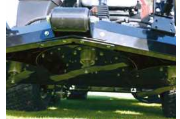
Low maintenance, direct drive hydraulic decks
